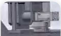
上限安全缸防止滑块下滑 Upper limit safety cylinder prevents the slider from sliding
